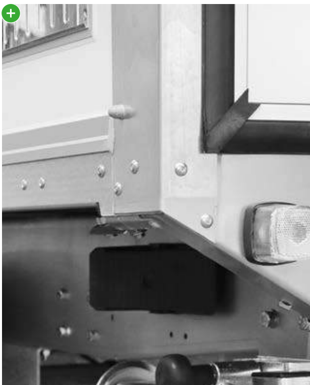
Corner angles Anodised aluminium corner angles riveted to the frame provide high torsional rigidity.
