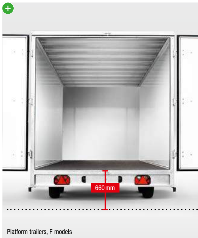
Loading heights For particularly easy loading and unloading of the van trailer, the F models have a low loading height from 660 mm. For the standard models it is up to 770 mm.
